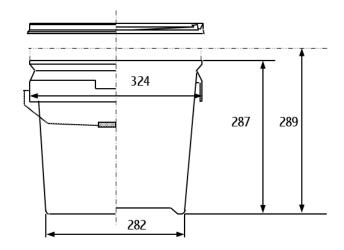
Measurements in millimetres
